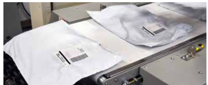
LABELS WITH BAR CODES & ADDRESS AUTOMATICALLY APPLIED
