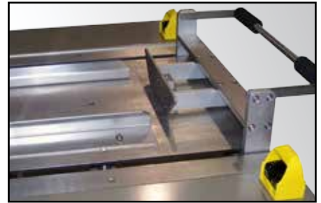
Manual Pusher Load station with palm buttons
