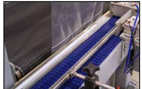
Powered Side Infeed Right angle conveyor with pneumatic pusher
